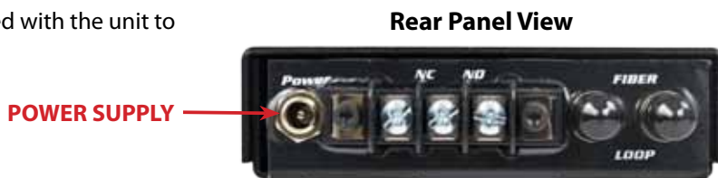
Terminal Block – A 3-pin terminal block is located in the back panel to provide a normally open (NO) and normally closed (NC) contact to trigger an external alarming device (siren, flashing light, etc.). This connection is a switch capable of carrying 3 amps (3A) of current.
