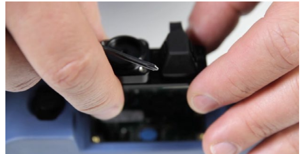
The power meter and VFL piece are offered as an easy-to-install option that's as simple as removing four screws.
