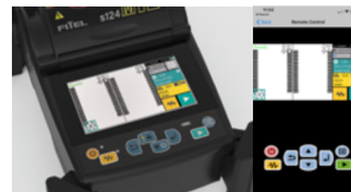
Touch panel and Wi-Fi network connectivity
